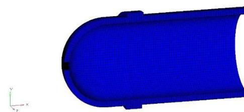
Fig:8.3:FEA model of FRP pressure vessel
